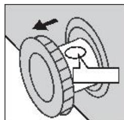
Rotate the drain dial 180 degree. This will let the water flow out in the tray.
